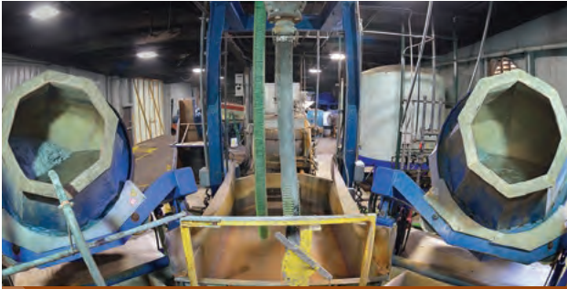
Mechanical finishing systems at Unimetal.
