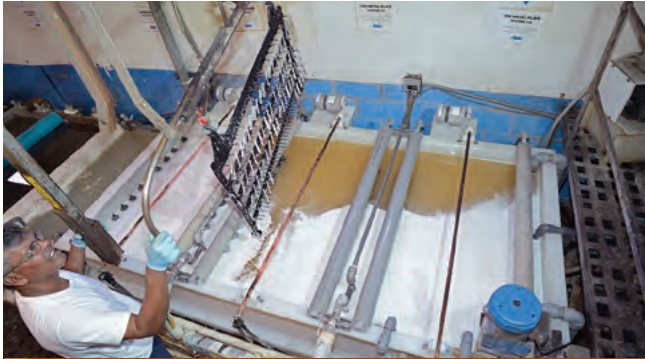
Gravity-hung copper-plated HF connectors are Miralloy plated.
