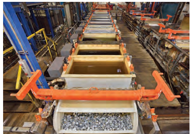
Automatic barrel chloride zinc line with 10 plating stations.
