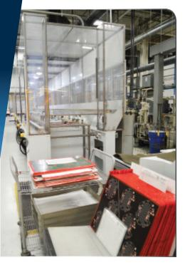
This automated line enables plating of about 1,500 PCB panels each week.
