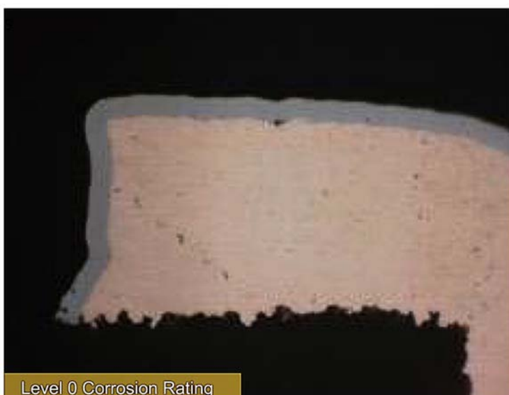
Figure 5: Cross-section of corrosion check after 40 minutes of dwell time in immersion Au bath.
