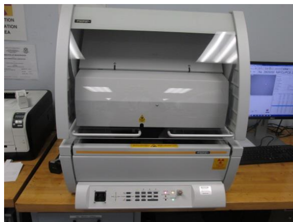
Figure 5: XRF used to measure plating thicknesses of the ENIG and EPIG test samples
