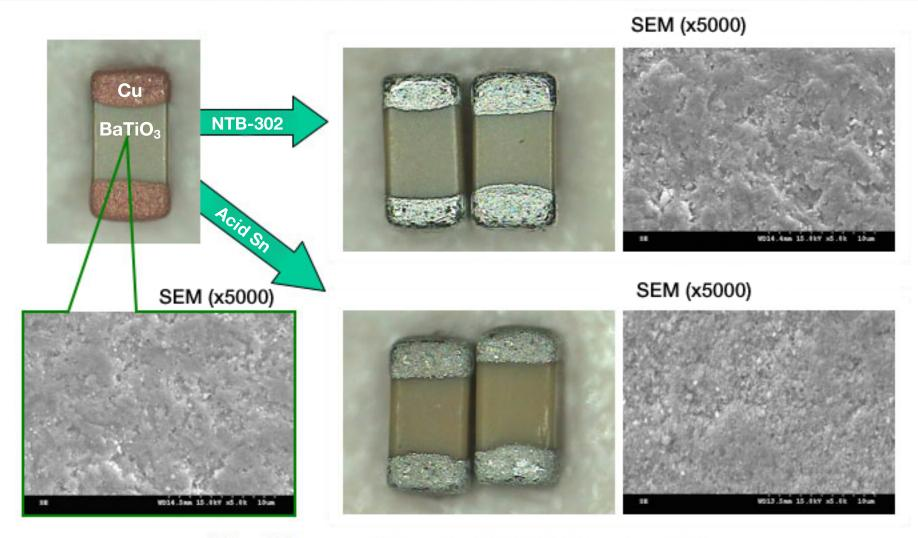
After 2 hours plating by NTB-302 and acid Sn NTB-302 shows no attack to the Barium Titante Ceramic
