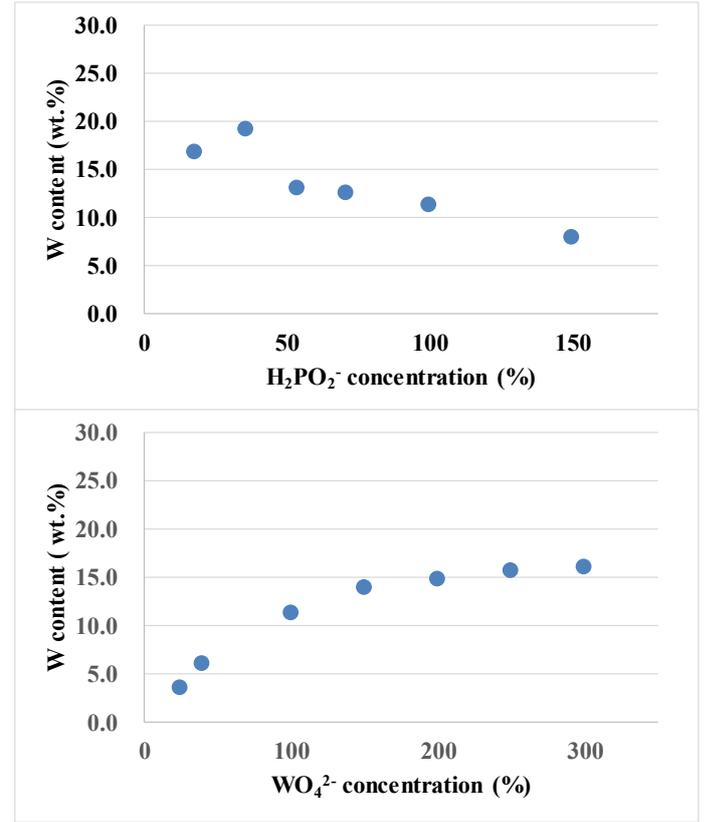
Fig. 1 W content of Co-W-P deposit (upper part: case of changing  $H_2PO_2^-$  concentration, lower part: case of changing  $WO_4^{2-}$  concentration)
