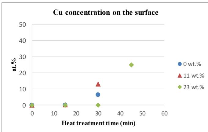
Fig. 3 Cu concentration on the surface by XPS analysis (Air, 400°C) (at.%)
