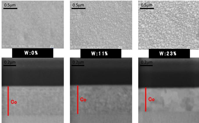
Fig. 2 FE-SEM (upper part) and FIB observation image (lower part) (Co-W-P deposit thickness: about 0.5 μm)
