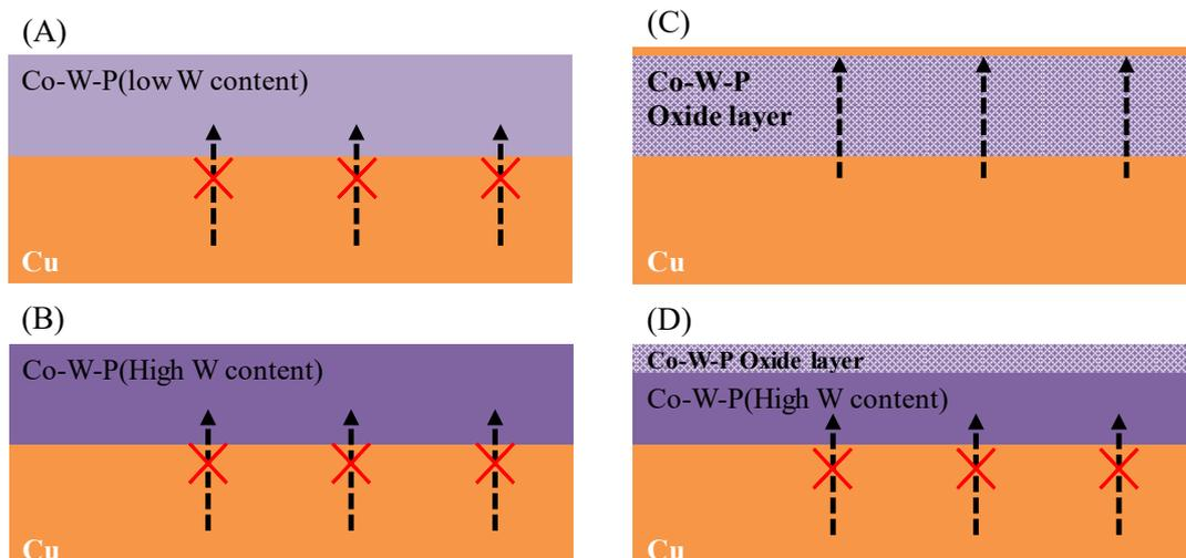
Fig. 5 Model of Cu diffusion occurrence (Heat treatment in N<sub>2</sub> : (A), (B), Air : (C), (D))
